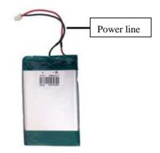
3 . Please plug power line into main board's battery socket.
