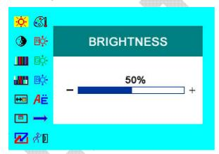
Press "</>"on the unit or " on the remote control to select item, eg. " , and it will be highlighted; and then press +/ - of the unit or / to adjust the favorite values. It shows picture mode specifications below the dialog box in DVI mode, but not in HDMI mode.
