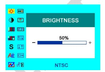
Press "</>"on the unit or " on the remote control to select item, eg. , and it will be highlighted; and then press +/ - of the unit or / to adjust the favorite values. It shows current picture format (NTSC&PAL) below the dialog box.
