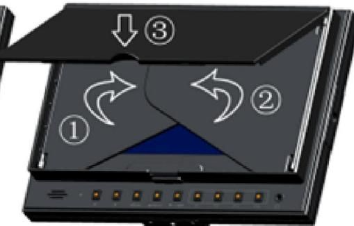
\* Do not press the edge in the under of the cover, otherwise it will result in open failure.
