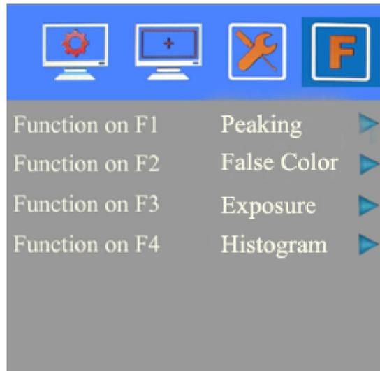
Functions of F1-F4 buttons can also be customized: Aspect Ratio, Check Field, Freeze Input, Center Marker, Underscan/Overscan, H/V delay, Color Bar, Screen Marker, Zoom, Peaking, False color, Exposure and Histogram.
