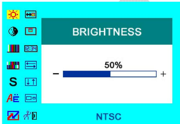
Press “</>” on the unit or “▲/▼” on the remote control to select item, eg. ☀, and it will be highlighted; and then press +/- of the unit or ◀/▶ to adjust the favorite values. It shows current picture format (NTSC&PAL) below the dialog box.
